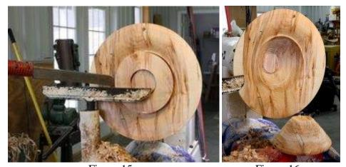
Figure 15 Figure 16 Begin hollowing the cap section of the hat. For the outback hat the outside shape should match the inside and be hollowed to  $\frac{1}{8}$ " wall thickness.
