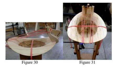
Apply a **small amount** of pressure by tightening the benders wing nut.
